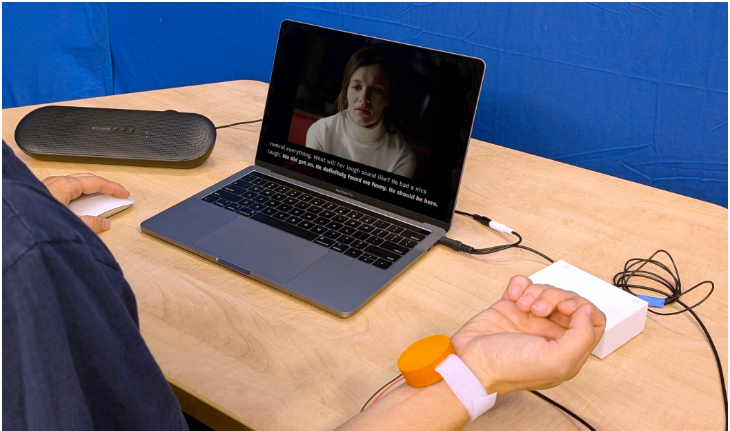
Fig. 2. To watch videos, participants would strap the voice coil to their arm, with the device face-down against the inside of their wrist. A laptop would drive both the haptic signals and an external speaker, that played the original sounds coming from the videos.
